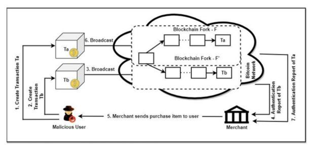
The recipient, who accepts the transaction without confirmation, gets duped when the attacker releases the previously mined block to the network, which invalidates the recipient's transaction and enables double-spending.
